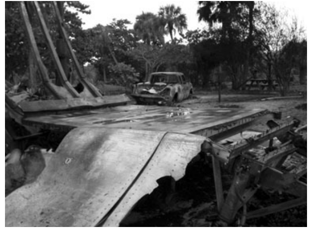
FIG. 4—The point of origin of the explosion in the rear of the semi-tractor trailer, on the right side of the photograph.
